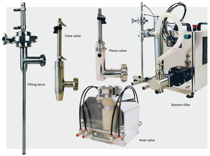
One of the many advantages with the Fillflex system is the possibility to control the whole filling process, down to the last detail. By equipping your filler with a pneumatic outlet valve, you can also handle "difficult" products with foaming properties or with solid particles.
