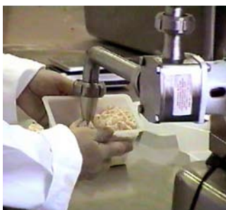
The impeller pump will not damage the product.
