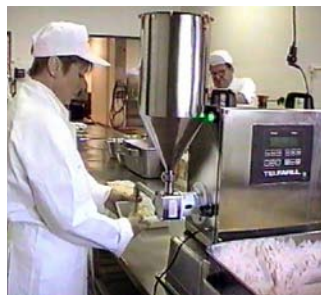
The salmon paté is poured in the feed hopper – simple, hygienic and easy to clean. (This work can also be automated with Telfafill Feed Pumps, if the client so wishes.)
